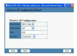
7. You have finished all basic configurations for WRT-416. Please press "Exit" to close this window. The WRT-416 will perform reboot if major changes are made. After reboot completes, the WRT-416 is ready to use.
